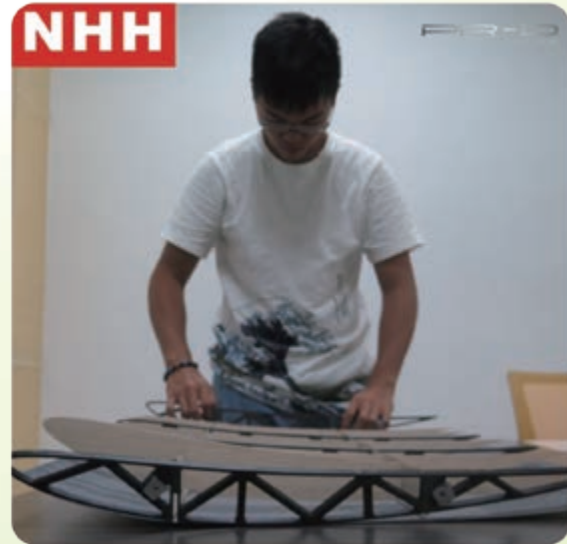
PolyU E-Formula Racing Team members are using carbon fiber PC composites developed and produced by the Group and using our 3D printing technology to assemble vehicle parts PolyU E-Formula Racing Team 隊員正在使用本集團自行研發及生產的碳纖維PC複合料並配合我們的3D打印技術組裝車輛部件
