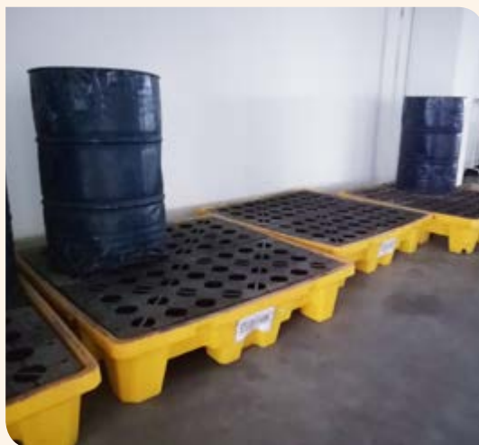
Industrial Waste Temporary Storage Area in the Factory Building and Special Card Board to Prevent Oil Leakage from the Tank 廠房內的工業垃圾暫存區及防止油品漏出油罐後造成污染的特製卡板
