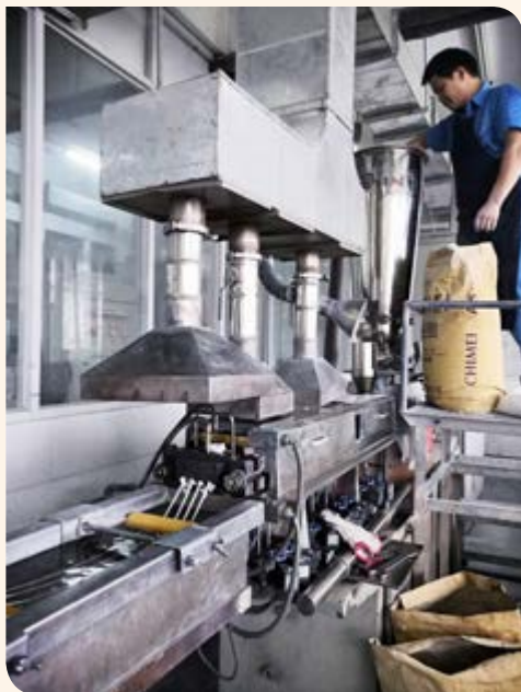
Dust Removal Equipment in the Feeding Process 投料工序中的除塵設備
